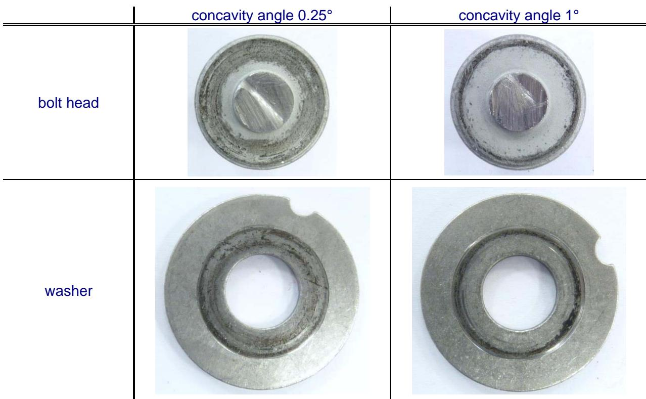
The evaluation of the measured effective diameter for the friction torque at the bolt head  $D_b$  shows a large standard deviation (**Annex 2**). For the mean values the results are:
