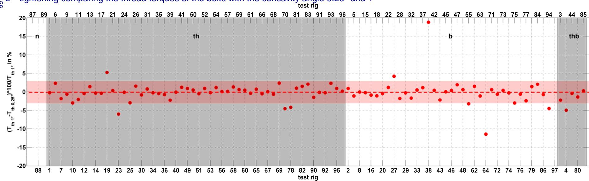
3<sup>rd</sup> tightening comparing the thread torques of the bolts with the concavity angle 0.25° und 1°
