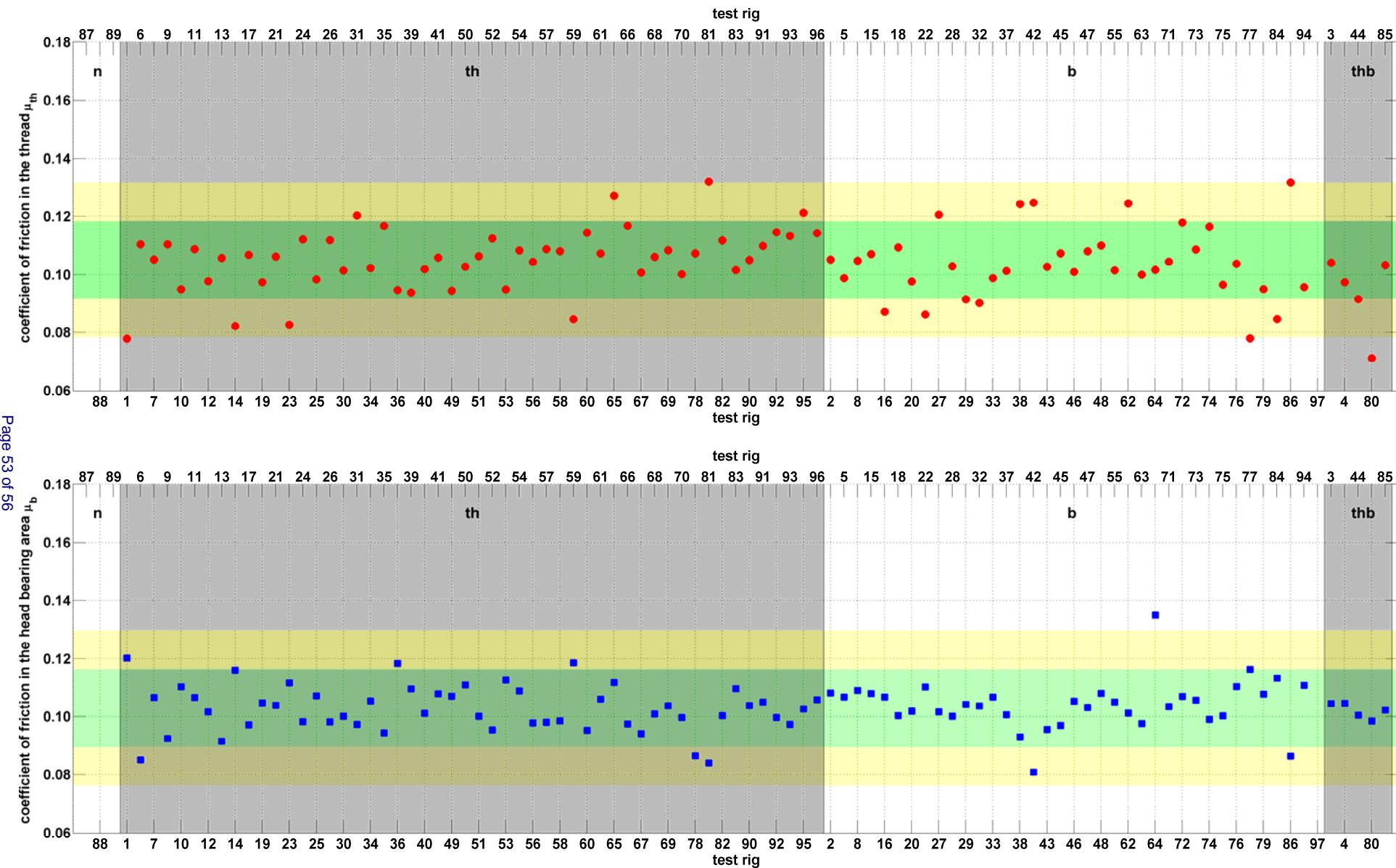
3<sup>rd</sup> tightening for bolts with concavity angle 1° and classification into the quality category
