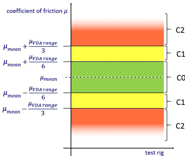
Figure 2: schematic diagram for the quality categories of the test rigs
