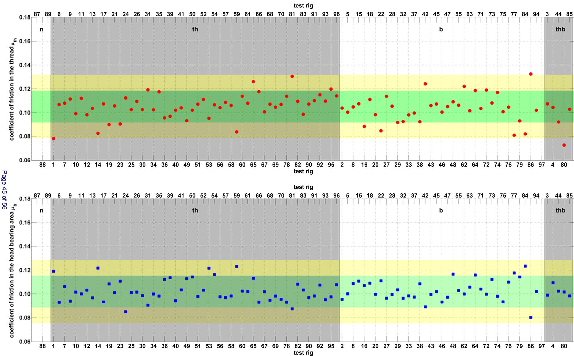
3<sup>rd</sup> tightening for bolts with concavity angle 0.25° and classification into the quality category
